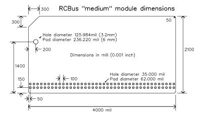
It is recommended that the mounting hole has a 6 mm diameter pad or a 6 mm unobstructed clearance for fixings
